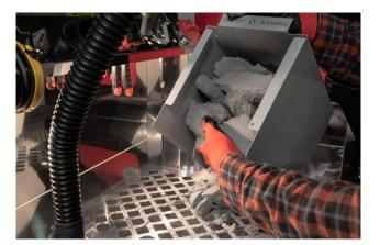
Thanks to the Chamber cover with large holes located on the worktop, you can easily push the unsintered powder through, while precleaning the print.
