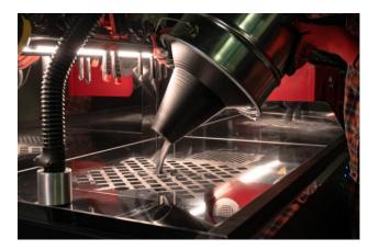
All the recovered powder is transferred to a sieving module and then goes into a metal container. Now it's ready to reuse
